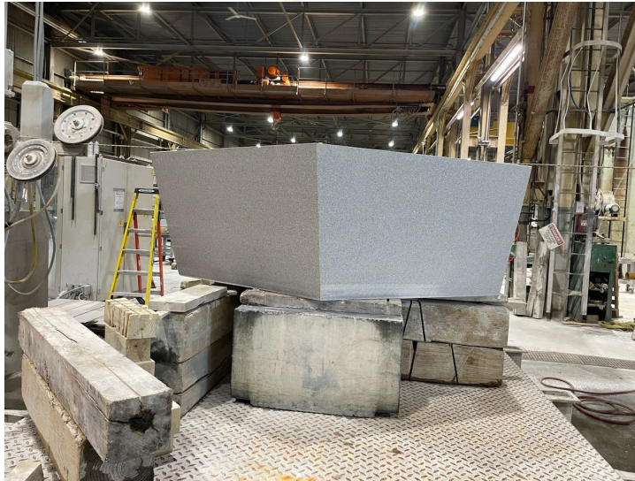
Base with two remaining cuts then headed to sandblast (Nov 23)
