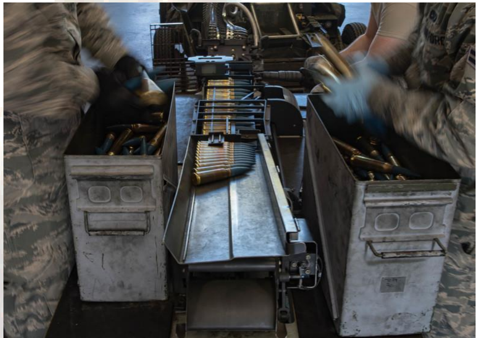
U.S. Air Force Airmen from the 1st Maintenance Squadron conventional unit, load 20 mm rounds on to a universal ammunition loading system at Joint Base Langley-Eustis, Virginia, May 1, 2018. The rounds are shot from an F-22 Raptor with an M16A2 20-millimeter cannon. (U.S. Air Force photo by Airman 1st Class Anthony Nin Leclerc) (Photo by Airman 1st Class Anthony Nin Leclerc)
