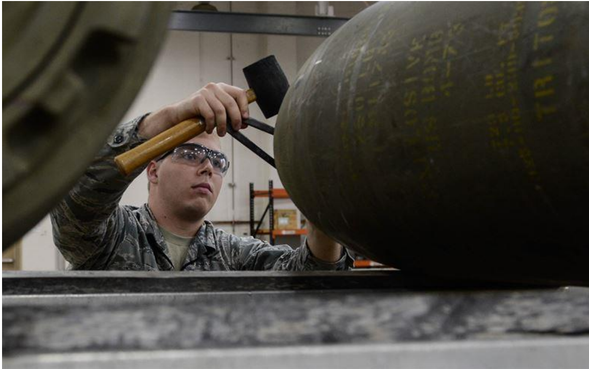
Airman 1st Class Brandon Kiernan, 2nd Munitions Squadron conventional maintenance technician, assembles an M-117 General Purpose Bomb at Barksdale Air Force Base, La., Nov. 8, 2017. The M-117 has been around since the 1950s. (U.S. Air Force Photo by Airman 1st Class Tessa B. Corrick)
