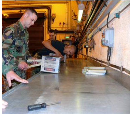
Senior Airman Jason Benchich (left) stuffs a chaff and flare canister with simulated munitions while Senior Airman Lester Delvalle (center) prepares a new canister at the start of a processing line April 21 at Royal Air Force Lakenheath, England. The Airmen are testing an Air Force Smart Operation for the 21st century initiative. The Airmen are assigned to the 48th Munitions Squadron. (U.S. Air Force photo/Tech. Sgt. Scott Wakefield)
