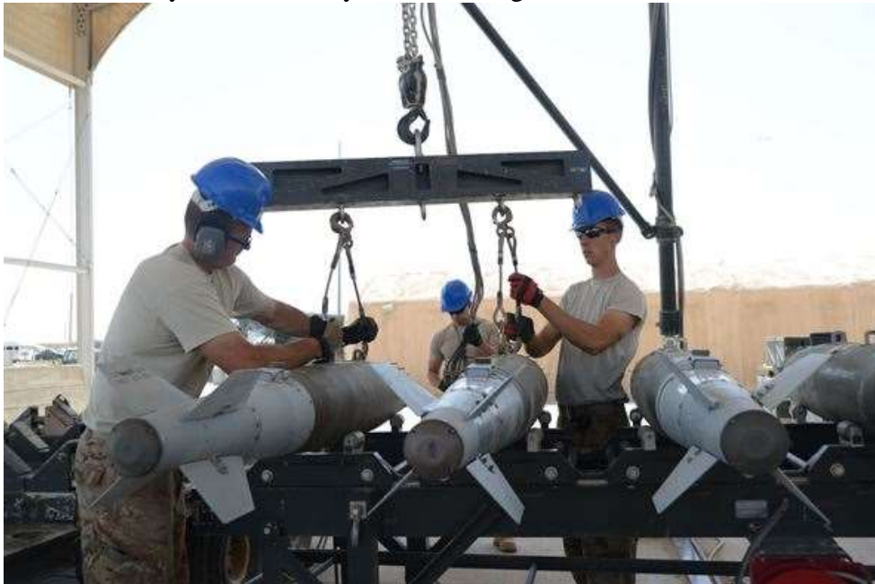
Tech. Sgt. Patrick Williams (left) and Senior Airman Brandon Graves attach GBU-38 bombs to a hoist that will be used with a munitions assembly conveyor to move the bombs during transport Aug. 14, 2014, at Bagram Airfield in support of Operation Enduring Freedom. Both men are currently assigned to the 455th Expeditionary Maintenance Squadron and both are reservists deployed from the 442nd Fighter Wing, Whiteman Air Force Base, Mo. (U.S. Air Force photo by Master Sgt. Cohen A. Young)
