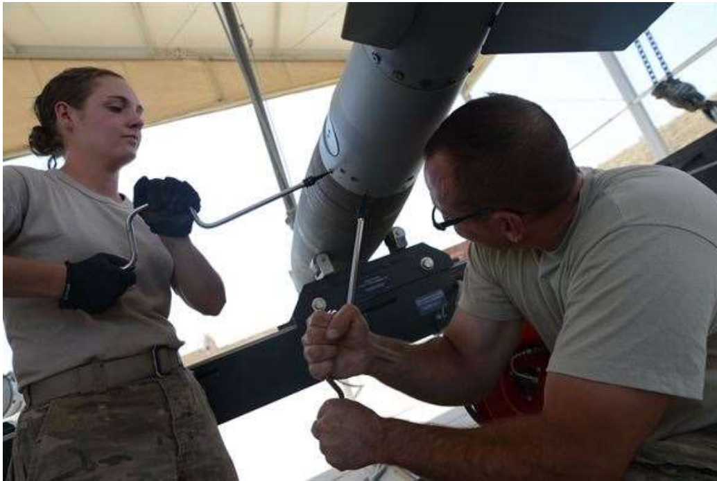
Airman 1st Class Casey Cain and Tech. Sgt. Patrick Williams tighten the screws on a GBU-38 during its construction while at Bagram Airfield, Afghanistan Aug. 14, 2014. The GBU-38 is a necessary part of the weapon system of the F-16C Fighting Falcon. Cain is a reservist deployed from Whiteman Air Force Base, Mo. Williams is a reservist deployed from the 442nd Fighter Wing in Missouri. (U.S. Air Force photo by Master Sgt. Cohen A. Young)
