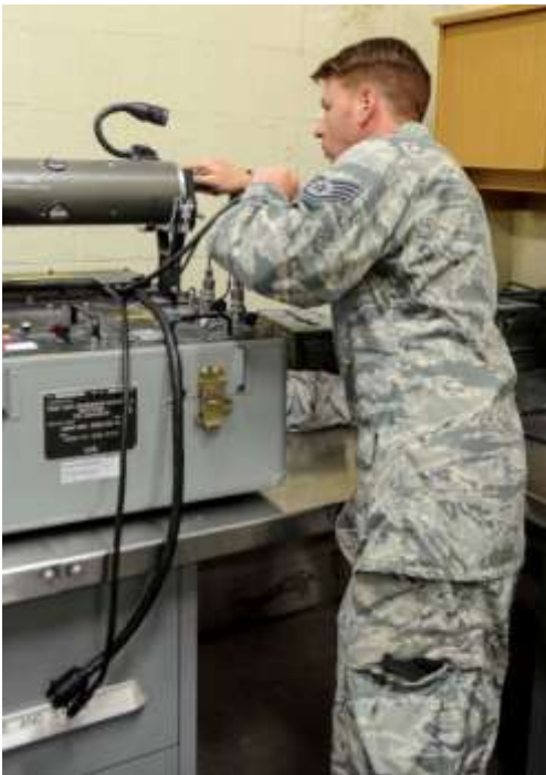
Staff Sgt. Travis Briese, 391st Fighter Squadron Munitions Flight equipment maintainer, connects the Captive Air Training Missile 9-M head to a TSU 4044 test set for trouble shooting.
