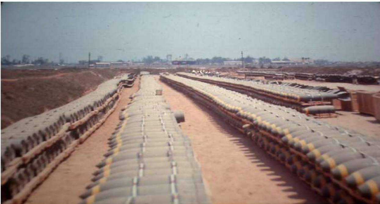
The 12-Man AMMO Crew in the back center right could build this many M117 750 lb GP Bombs in Four Days. Four troops breaking-out and pulling plugs, two troops jamming boosters, two troops lugging, two troops prepping fins, two troops hanging fins to start.....and the others caught up with the fin crew to finish it off. They were the BEST I EVER SAW.
