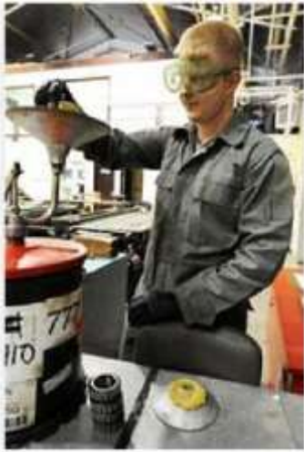
Airman 1st Class Cristian Grady, 35th Maintenance Squadron, packs bearings for a Munitions Handling Unit 141 trailer that is due for a 720 day inspection here, Jan. 17. Grady, a Cedar Rapids, Iowa native has been working as a mission support equipment crew member since November 2010. (U.S. Air Force photo/Airman 1st Class Kia Atkins)
