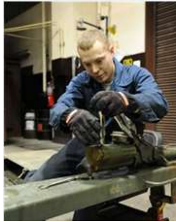
Senior Airman Quintin Chandler, 35th Maintenance Squadron equipment maintenance crew chief, bleeds brakes on a Munitions Handling Unit 141 trailer that is due for a 720 day inspection here, Jan. 17. The MHU-141 trailer is a four-wheeled, two axle automotive type steering vehicle capable of transporting loads up to 5,700 pounds. (U.S. Air Force Photo/Airman 1st Class Kia Atkins)
